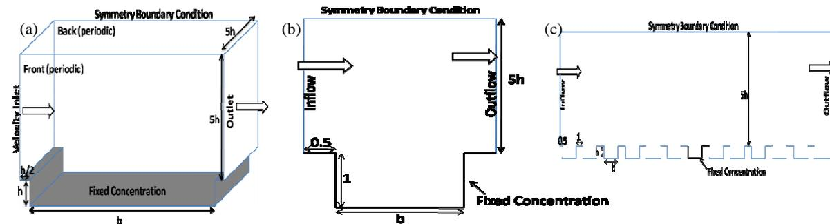
Figure 1. (a) Computation domain of the LES; (b) averaged two-dimensional computational domain in the LES; and (c) 13-street-canyon computational domain in the  $k-\epsilon$  turbulence model
