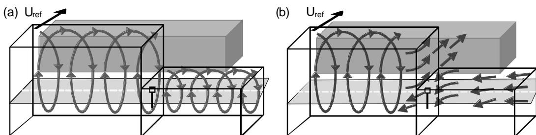
Figure 6 - Schematic diagram illustrating (a) the helicoidal flow within North Lane for oblique background winds approximately within the sector  $\approx 175^\circ < \theta_{\text{hlds}} < 240^\circ$  when in-street flow is being channelled towards the intersection ( $210^\circ < \theta_{\text{in-st}} < 300^\circ$ ), and (b) the convergence of flow within North lane when the in-street channelling recorded is away from the intersection ( $30^\circ < \theta_{\text{in-st}} < 120^\circ$ ).
