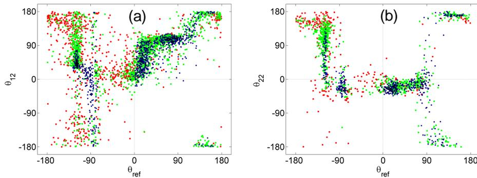
Figure 3. 15-minute mean wind direction ( $\theta_{ij}$ ) against roof-top wind direction ( $\theta_{ref}$ ) for in-street sonics, (a) Site 1 lower, (b) Site 2 lower. Thresholds of roof-top wind speed ( $U_{ref}$ ):  $\blacklozenge U_{ref} < 1.1 \text{ m s}^{-1}$ ,  $\blacklozenge 1.1 \leq U_{ref} \leq 2.5 \text{ m s}^{-1}$ , and  $\blacklozenge U_{ref} > 2.5 \text{ m s}^{-1}$ .
