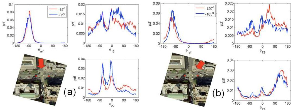
Figure 4. Wind direction pdfs for 1 hour segments of 10 Hz data at the DAPPLE intersection sites for  $\theta_{ref}$  wind sectors a)  $-75^\circ \leq \theta_{ref} \leq -105^\circ$  b)  $-105^\circ \leq \theta_{ref} \leq -135^\circ$ . Top left: roof-top wind direction pdf where legend indicates mean flow direction, bottom left: site layout with arrow pointing in the direction of flow, top right: site 1 (lower sonic) and bottom right: site 2 (lower sonic).
