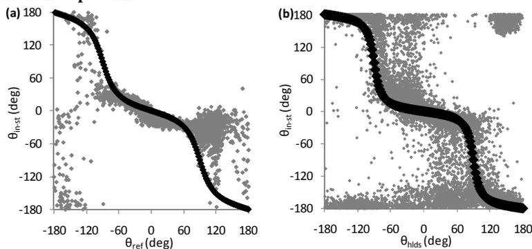
Figure 2 Plot showing the relationship between the reference wind direction  $\theta_{ref}$  and the in-street wind direction for (a) DAPPLE site 3 (b) the North Lane canyon, Leeds. The gray symbols are 15-minute averages of the measured data and the black symbols the fitted model of (Dobre *et al.*, 2005).
