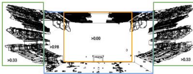
Porosity thresholds used to create the mesh
