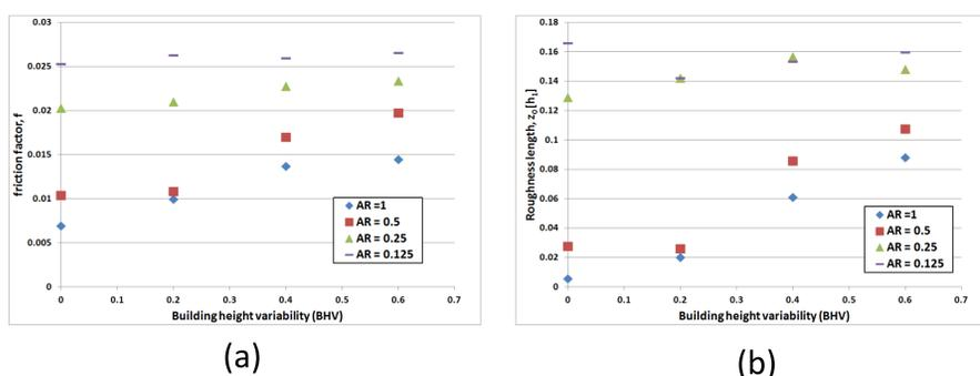
Fig. 2. (a) Friction factor  $f$  and (b) roughness length  $z_0$  plotted against building height variability (BHV) for street canyons of different aspect ratio AR.
