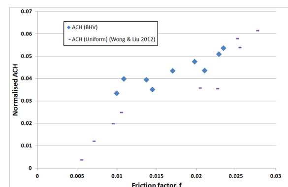
Fig. 4. Normalized air exchange rate ACH plotted against friction factor  $f$ .
