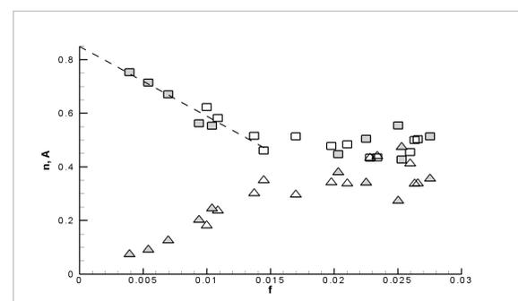
Fig. 3. Empirical coefficients in Equation 2 expressed as functions of friction factor  $f$ . A: square;  $n$ : triangle; LES over uniform street canyon: filled symbols; LES over 2D street canyon with BHV: empty symbols; The linear regression  $n = -26.1f + 0.85$  with  $R^2 = 0.936$  for  $f < 0.015$ : dashed line.
