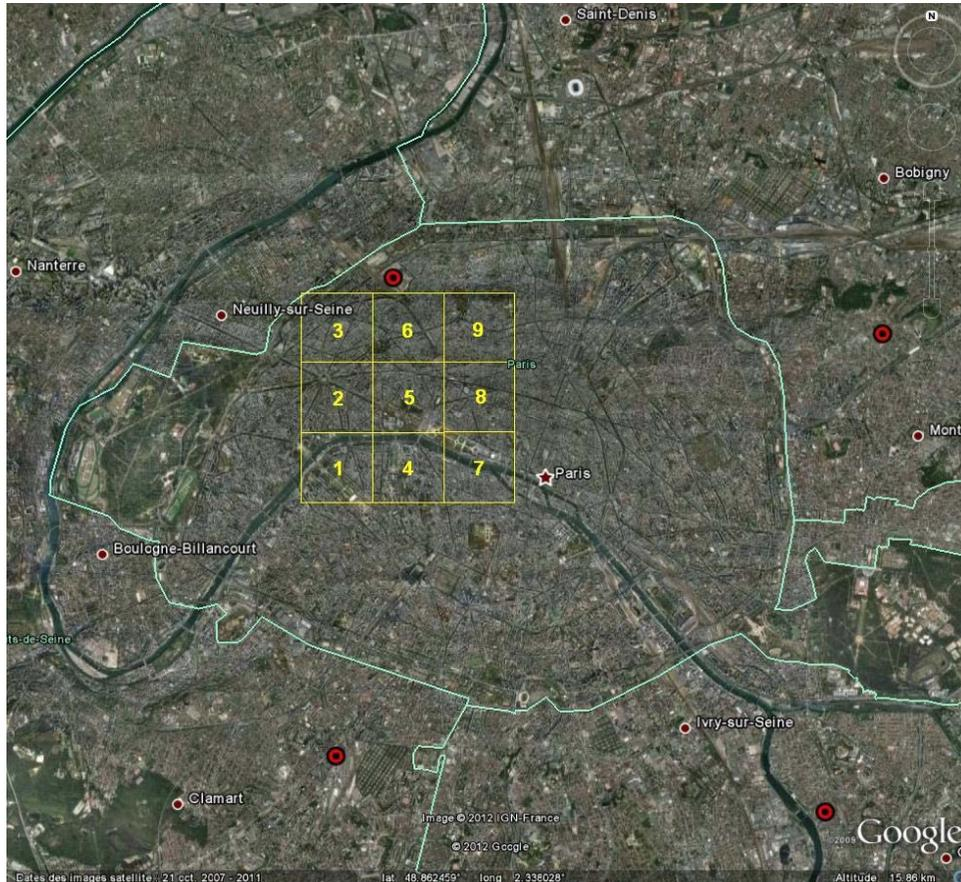
The red dots are meso-model grid nodes where wind, temperature and humidity vertical profiles are extracted for the urban mass-consistent flow diagnostic
