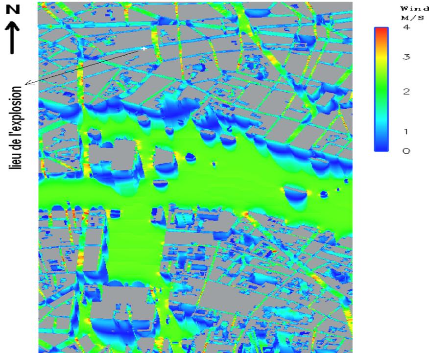
In the “free from buildings” areas, the velocity is a bit less than  $3 m.s^{-1}$ , consistent with the meso-scale prediction. On the contrary, in the “influenced by the buildings” areas, wind velocity is weaker, around  $1 m.s^{-1}$ , except in the N-S streets where the velocity can reach more than  $4 m.s^{-1}$
