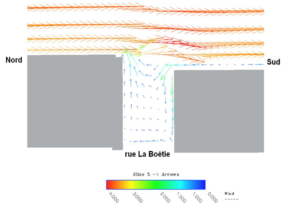
This zoom shows the flow complexity inside the streets, especially for streets perpendicular to the wind axis where the air flux near the ground is opposed to the wind N-S main direction due to a vortex forming induced by the flow above the roof level (spiral motion of the air in these W-E streets)
