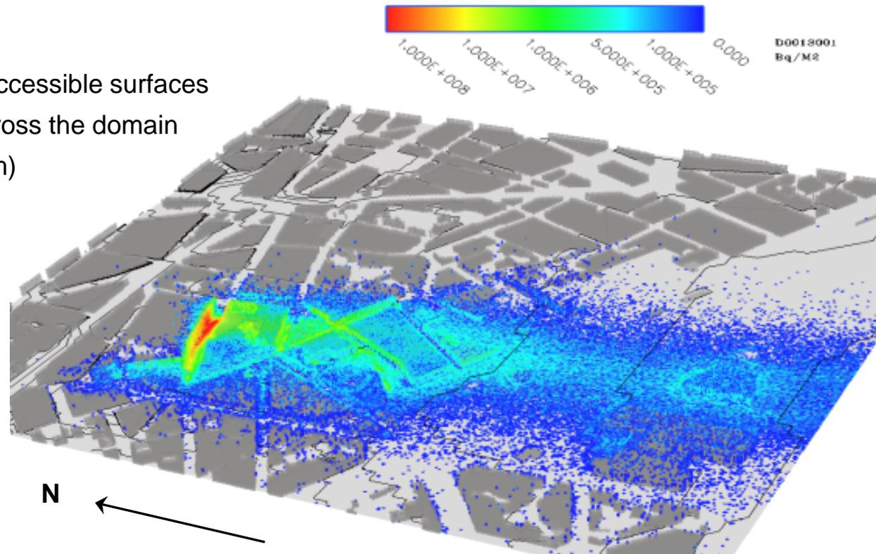
In the exercise, we did not evaluate infiltration inside the buildings although PSPRAY can do it. Obviously, it is the most important where deposition on façades is the highest!
