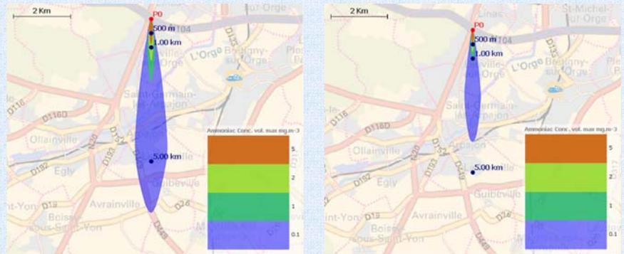
Fig. 1. NH<sub>3</sub> max. concentration (in mg.m<sup>-3</sup>) without (left) and with (right) chemical reactivity.
