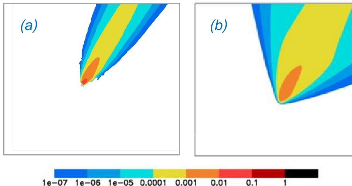
*A comparison of inverse plumes for receptor 1 using (a) 3D CFD model (PANEPR), (b) 3D analytical model along plane of release height above the ground*
