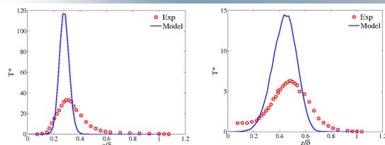
Comparison of vertical profiles at increasing distance from the source in  $Fr=4, R=2$ ; simulations without additional spread (Model I); (a)  $x/\delta=0.463$ ; (b)  $x/\delta=1.852$ .
