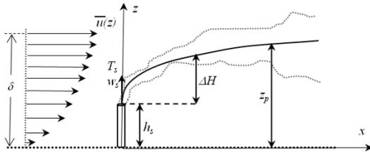
An adiabatic atmospheric boundary layer flow was obtained by means of vortex generators and a roughness distribution placed, respectively, at the wind tunnel inlet and on the ground. The measurements of velocity are performed through a X-wire anemometer.
