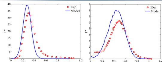
Comparison of vertical profiles at increasing distance from the source in  $Fr=4, R=2$ ; simulations with additional spread (Model II); (a)  $x/\delta=0.463$ ; (b)  $x/\delta=1.852$ .
