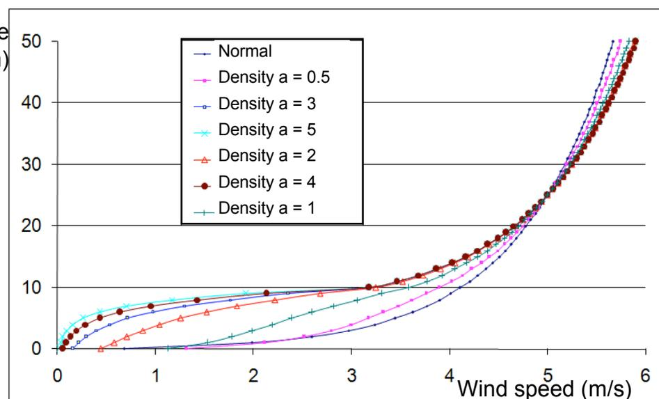
Influence of the canopy density parameter on a log wind profile shape with 5m/s at 25m (canopy height 10m, roughness 0.15m)
