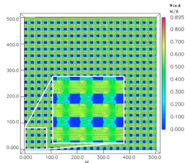
Micro domain calculation for west wind, wind field intensity and streamlines at a height of 5m
