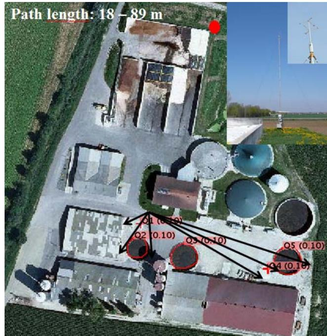
Figure 1. Sources, laser paths, picture and location (red dot) of the ultrasonic anemometer at the biogas plant (north orientated)
