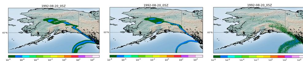
Figure 5.  $\text{SO}_2$  total column concentration ( $\text{kg m}^{-3}$ ). FLEXPART left, HYSPLIT middle, PUFF right.
