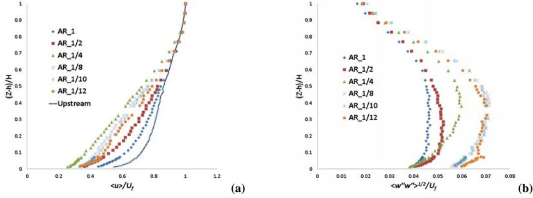
Figure 3. Vertical profiles of normalized (a) mean streamwise velocity and (b) vertical velocity fluctuation at various aspect ratios tested.
