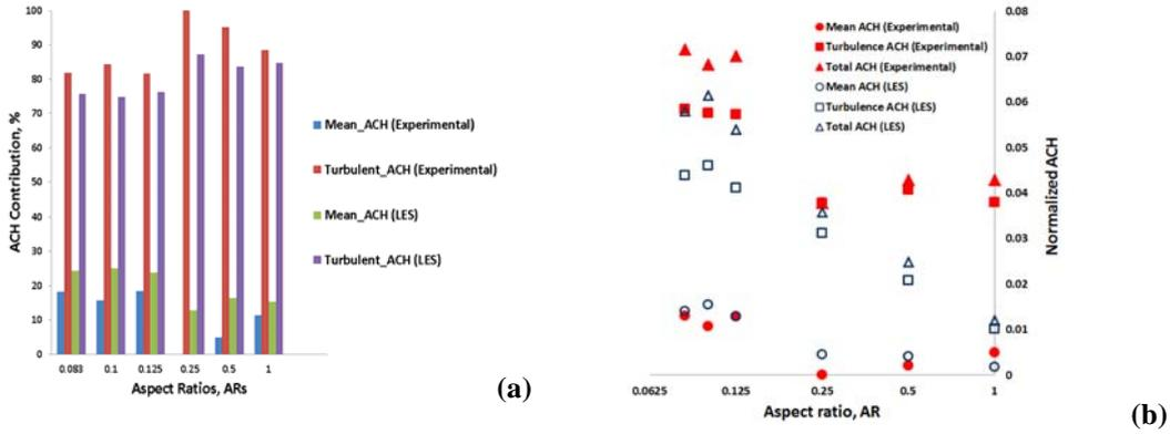
Figure 4. (a) Decomposed air exchange rate (ACH) and (b) dimensionless ACH plotted against ARs.
