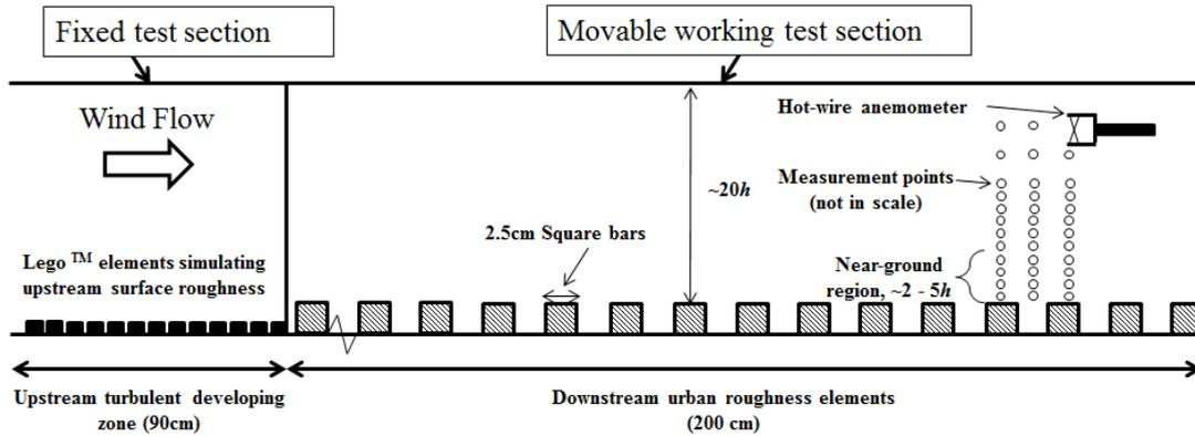
Figure 2. Schematic of the instrumentation details.
