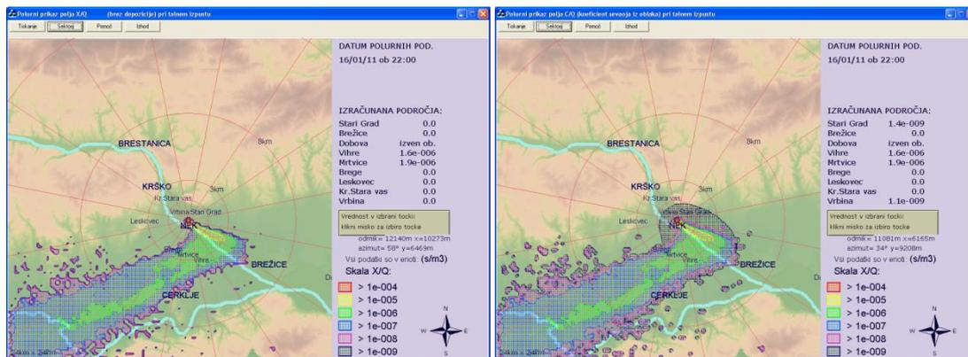
Figure 2. A comparison for a ground-level release.  $X/Q$  is shown on the left and  $C/Q$  on the right. The greatest difference is on the windward side, where  $X/Q = 0$ . There is no difference at the edges, because the cloud stays close to the ground.
