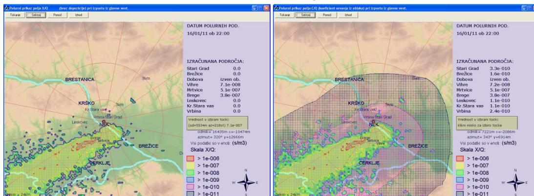
Figure 1. A comparison for a release from the main ventilation. In the example X/Q is shown on the left and C/Q on the right. The greatest difference is at the edges of the cloud, where most of the cloud is at a higher altitude.
