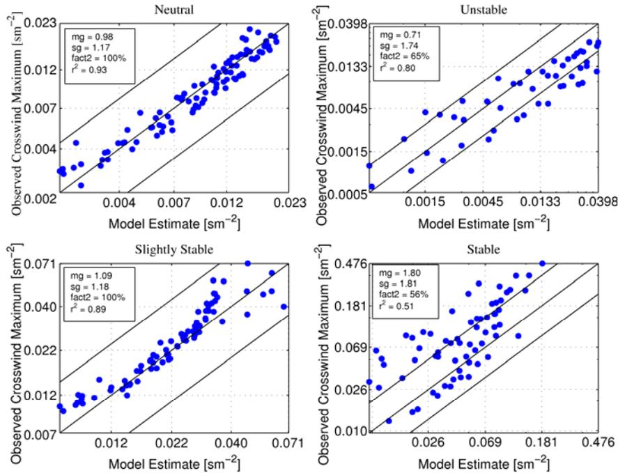
Figure 2: Comparison of mixed-wake model crosswind maximum concentrations with NRTS08 crosswind maximum concentrations. The model was run with  $\sigma=1.3$ . The model performance is similar to the source-shift, except during day 2, when the model performs better than the source-shift.
