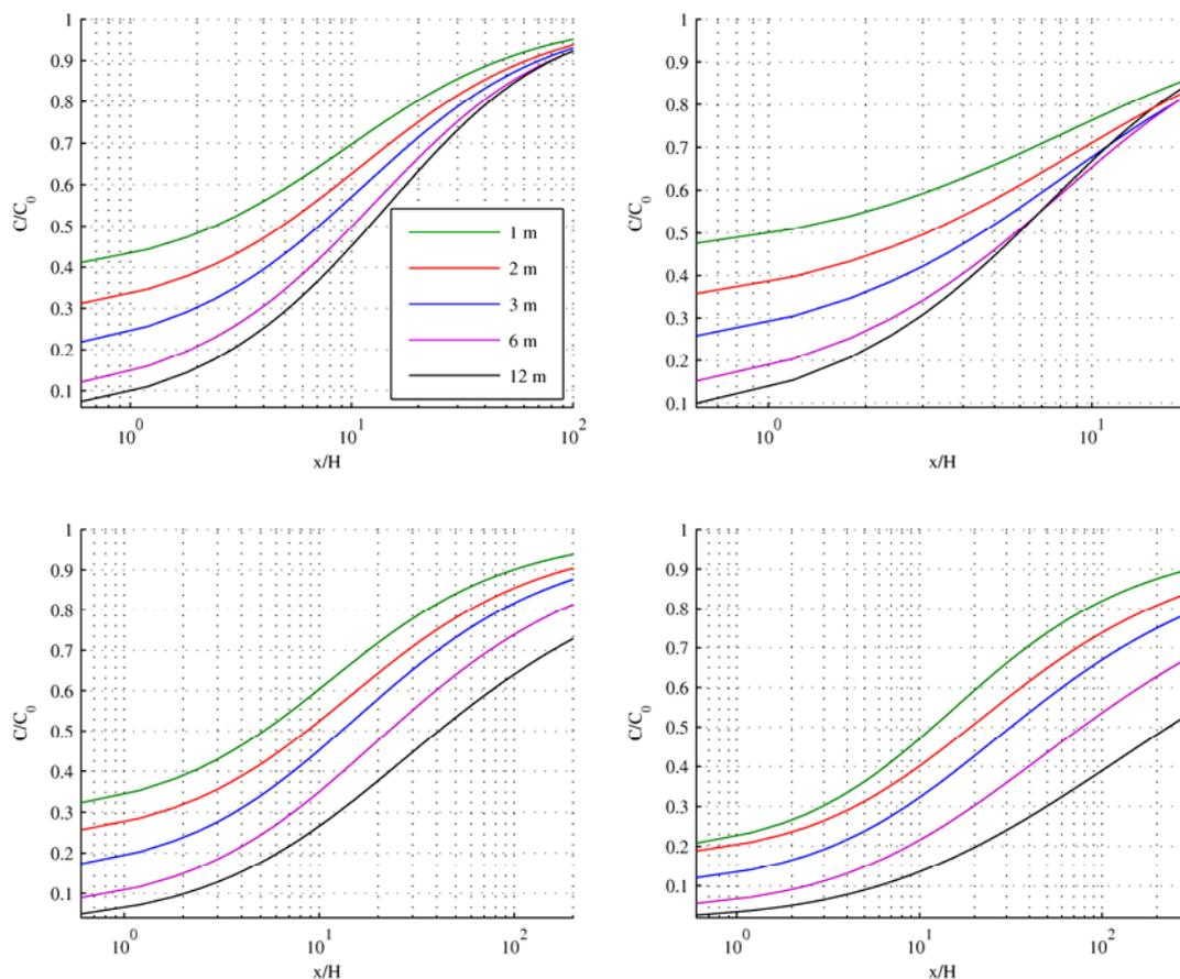
Figure 3: Sensitivity of mixed-wake model predicted concentrations to changes in barrier height vs. downwind distance for meteorology representing neutral (top left), unstable (top right), slightly stable (bottom left), and strongly stable (bottom right) atmospheric conditions. The barrier height,  $H$ , takes values of 1 m, 2 m, 3 m, 6 m, and 12 m. Note the different horizontal scale.
