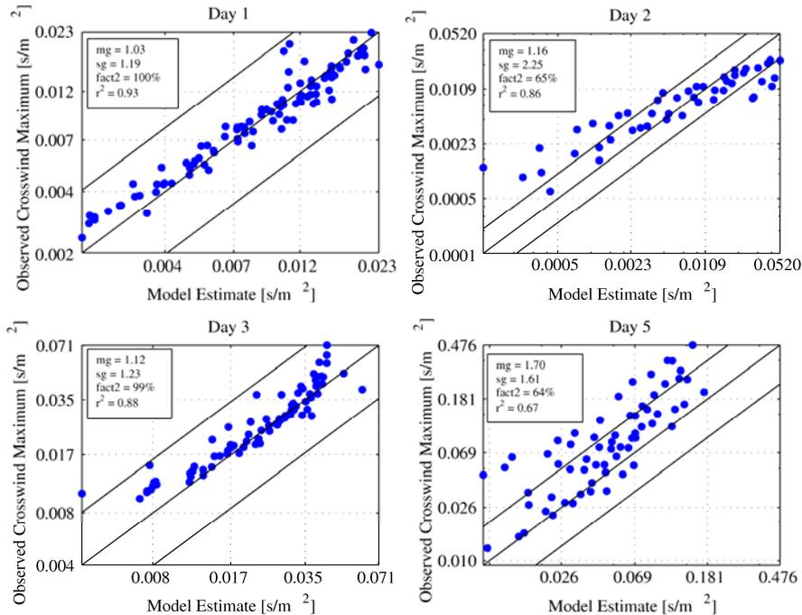
Figure 1: Scatterplots comparing the source-shift with mean crosswind maximum concentrations observed during NRTS08. The model was run with  $\sigma=0.5$ . The model performs best during neutral conditions and worst during very stable conditions. The model slightly overestimates during day 3, and tends to underestimate concentrations far from the barrier.
