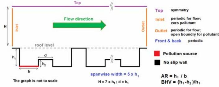
Figure 1. Computational domain and boundary conditions.
