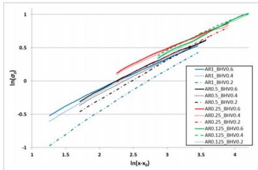
Figure 5. Vertical dispersion coefficient against streamwise distance from pollutant source in logarithmic scale.
