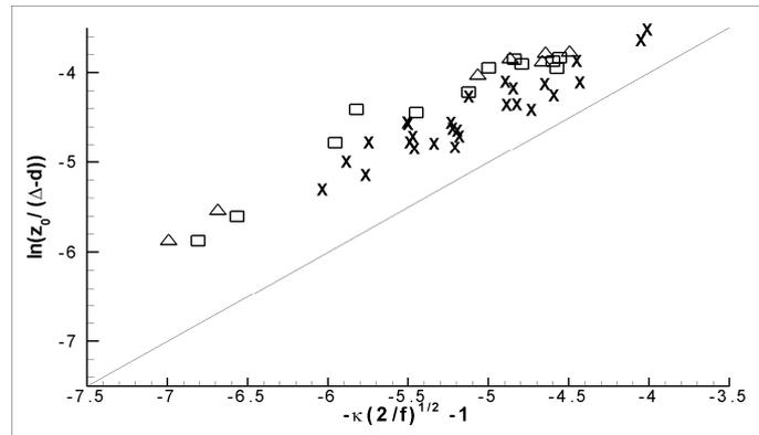
Figure 2. Roughness length scale  $z_0$  plotted as a function of the friction factor  $f$ . LES over uniform street canyon: square; LES over 2D street canyon with BHV: triangle; and wind tunnel experiment by Hagishima *et al* (2009): cross. Solid line is the theoretical solution  $E = 0$ .
