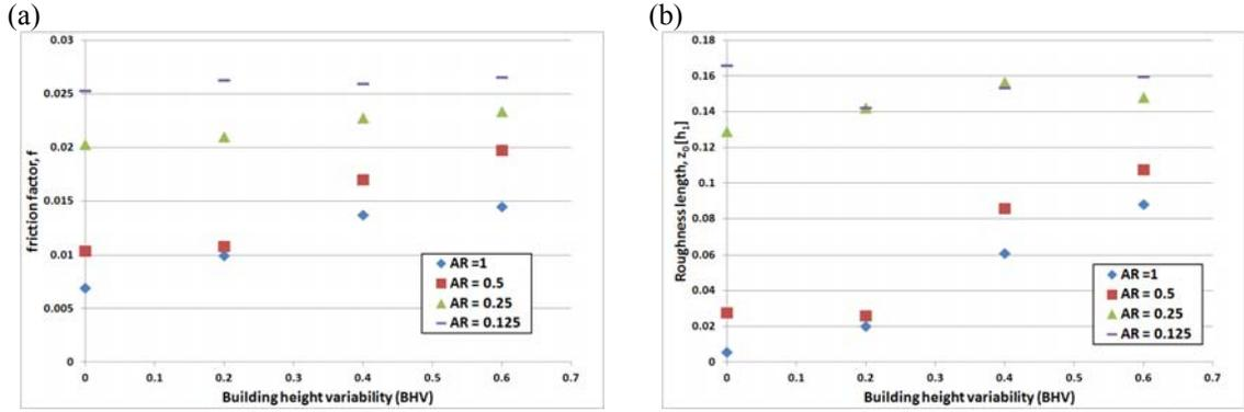
Figure 3. (a) Friction factor  $f$  and (b) roughness length  $z_0$  plotted against building height variability BHV for street canyons of different aspect ratio AR.
