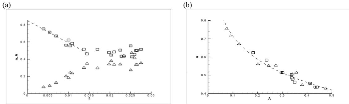
Figure 6. (a) Empirical coefficients in Equation 2 expressed as functions of friction factor  $f$ . A: square;  $n$ : triangle; LES over uniform street canyon: filled symbols; LES over 2D street canyon with BHV: empty symbols; The linear regression  $n = -26.1f + 0.85$  with  $R^2 = 0.936$  for  $f < 0.015$ : dashed line.
