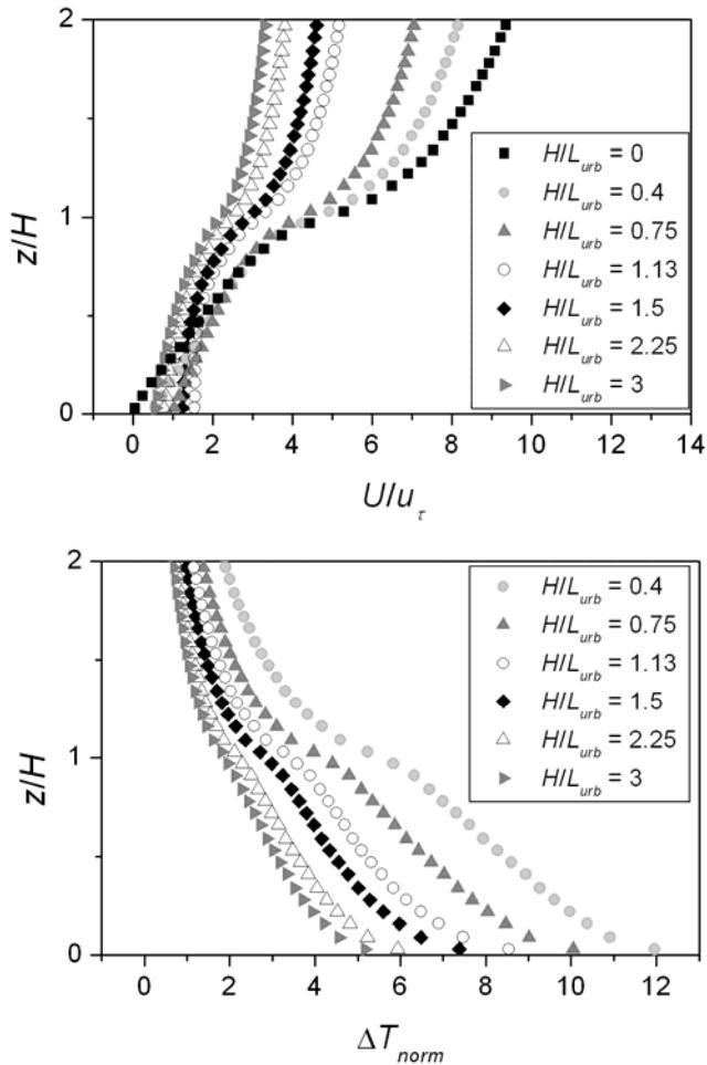
Figure 3. Vertical profiles of spatially-averaged streamwise velocity and  $\Delta T_{norm}$  for cases with the different  $H/L_{urb}$ .
