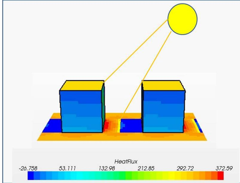
Figure 1. TUF3D surface sensible heat flux distribution corresponding to 10 am (zenith angle 30°) during the Equinox at the Equator.
