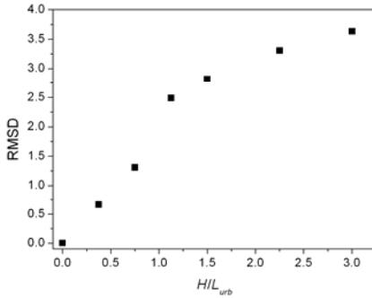
Figure 4. RMSD comparing average streamwise velocity vertical profiles of cases with different  $H/L_{urb}$  with the neutral case ( $Q_h = 0$ ). Values are compared from  $z/H = 0$  to  $z/H = 2$ .
