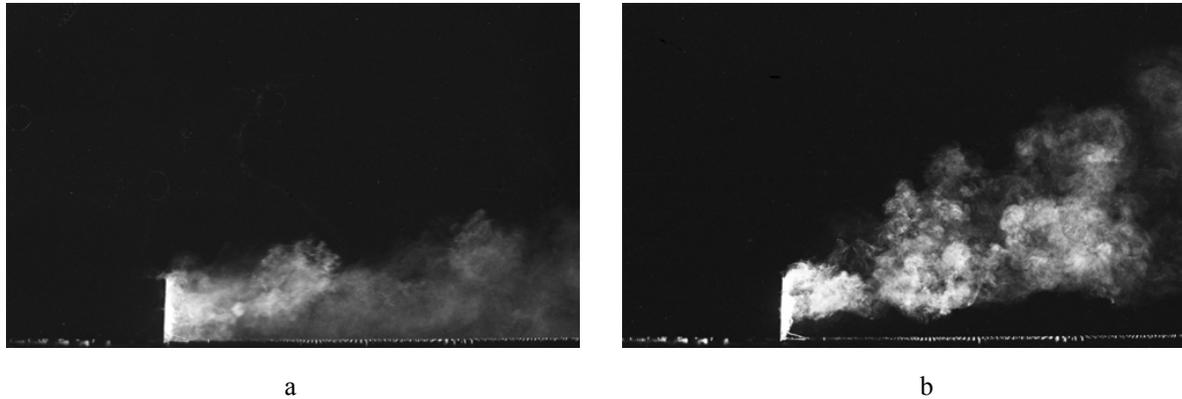
Figure 1. Flow visualisation of plume discharges from building wake with (a) neutral and (b) high buoyancy (Hall et al 1980).
