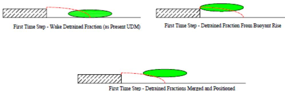
Figure 2. Schematic of model for buoyant puff detrainment from a building wake.
