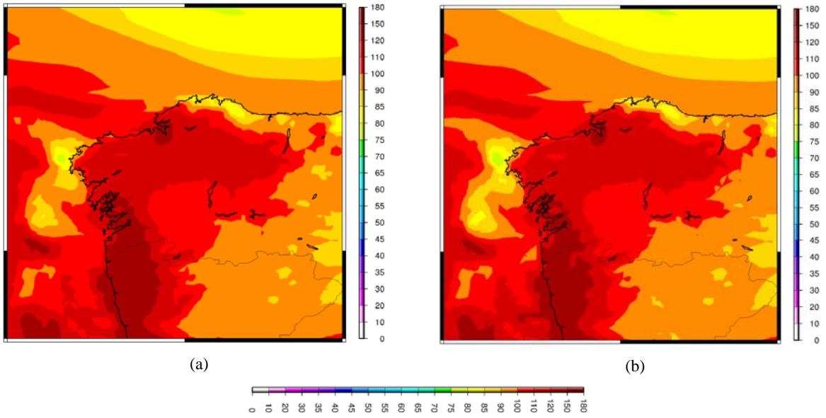
Figure 4.  $O_3$  glc (in  $\mu\text{g}/\text{m}^3$ ) at 12:00 UTC, from the CHIMERE simulations using July, 18<sup>th</sup> 2002 meteorological conditions, with (a) 2002 EMEP emissions inventory; and (b) 2008 EMEP emissions inventory.
