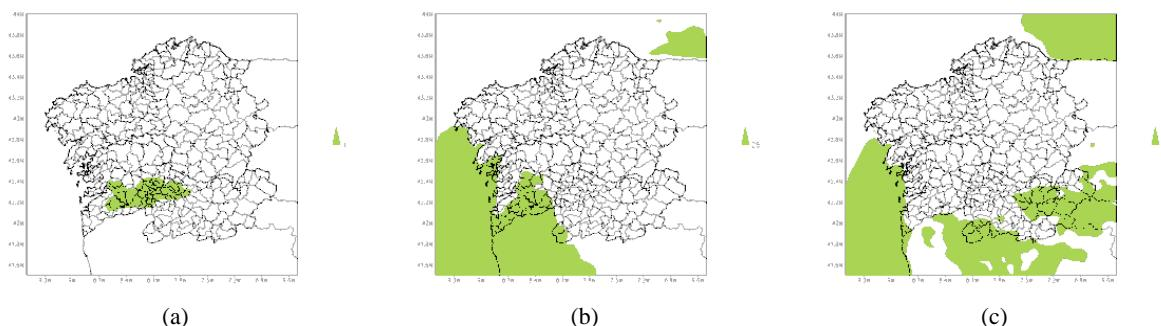
Figure 3. Optimal air quality network design: Areas with exceedances in the  $\text{O}_3$  thresholds: (a) report to people; (b) health; (c) vegetation (AOT40).
