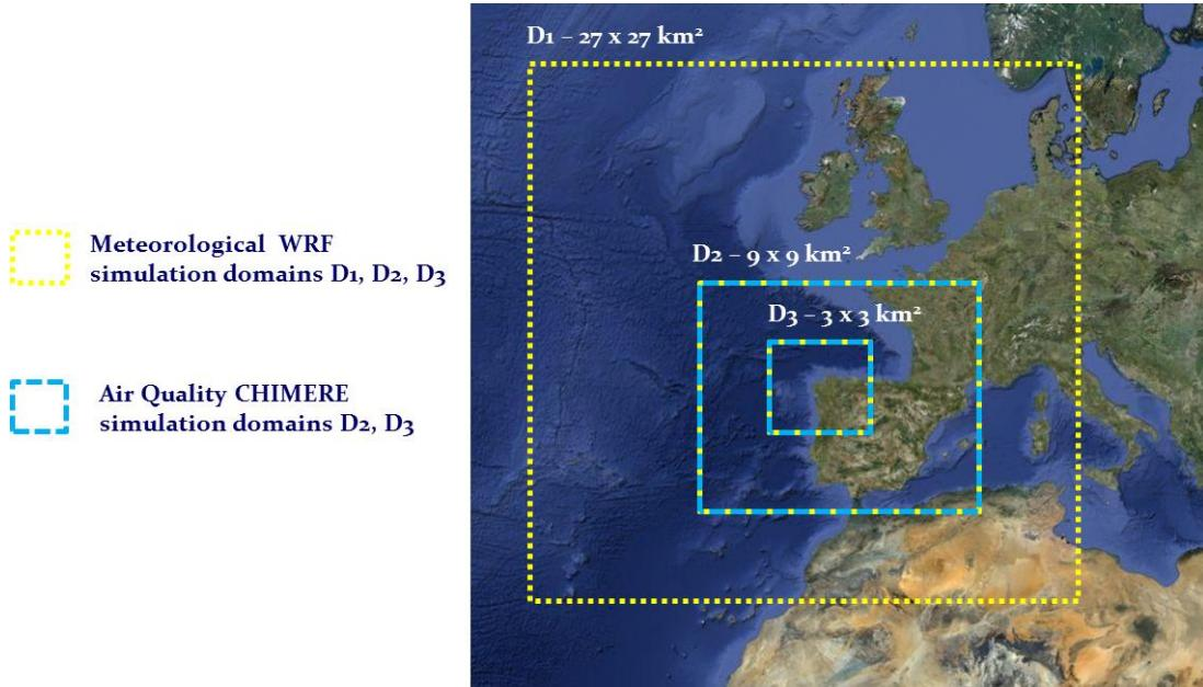
Figure 1. Simulation domains and grids applied in WRF-ARW meteorological model, and CHIMERE air quality model.
