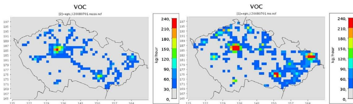
Figure 2. VOC emissions into first model layer at 7 UTC July 1st. TNO/MEGAPOLI emissions (right) include small point sources, area sources and transport. Czech national emissions REZZO (left) include local heating, solvent use and transport.
