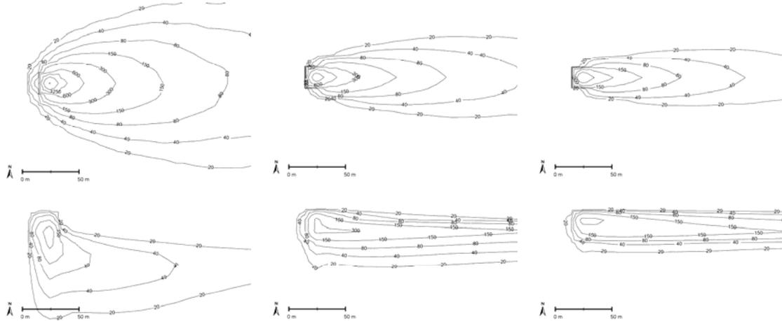
Figure 2. Comparison of computed concentrations from a point source near ground (top) and a tunnel portal (bottom) for three different wind speeds (left:  $1 \text{ m s}^{-1}$ ; middle:  $3 \text{ m s}^{-1}$ ; right:  $5 \text{ m s}^{-1}$ )
