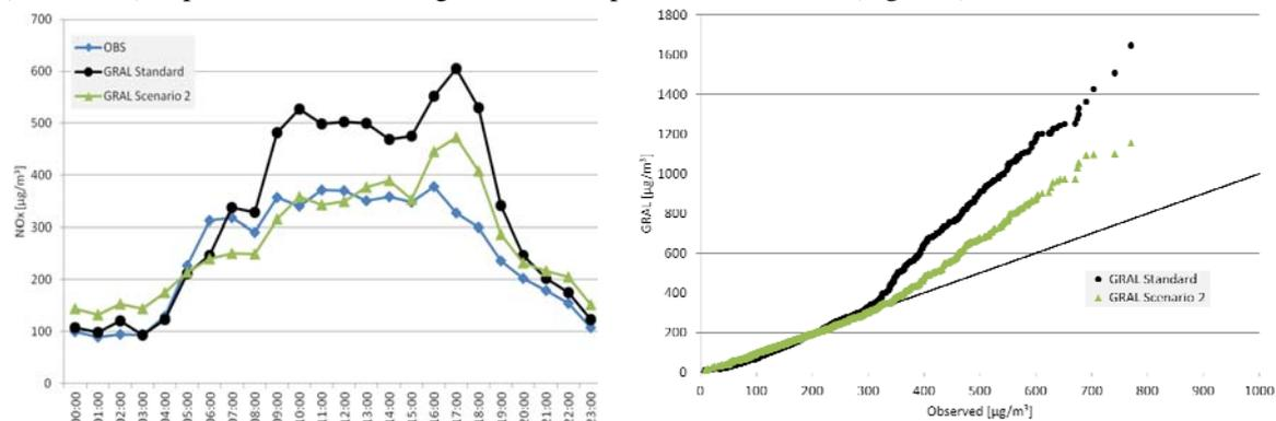
Figure 4. Comparison of observed and modelled average diurnal NO<sub>x</sub> concentrations (left); Quantile-quantile plot (right)
