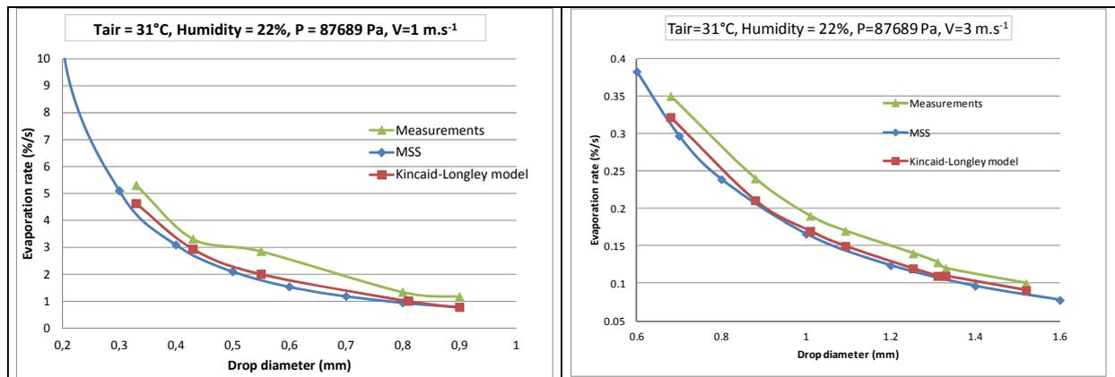
Figure 1: Evaporation rate of droplets in different conditions
