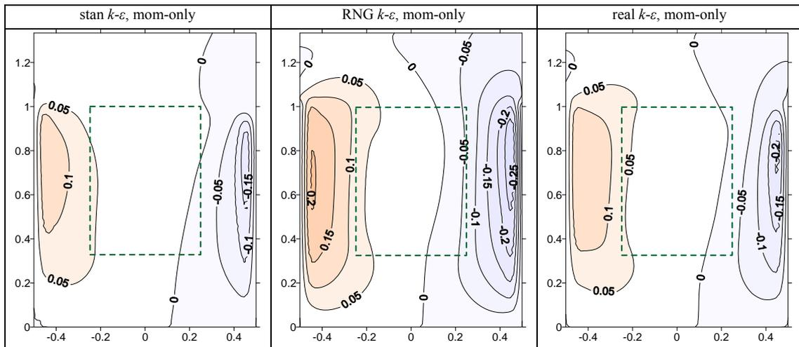
Figure 2. Simulated normalized vertical velocities  $U_3/U_H$  in the vertical plane at  $x_2/H = 0.5$  (Figure 1) with the extra terms in the momentum equations only (Equation 1).
