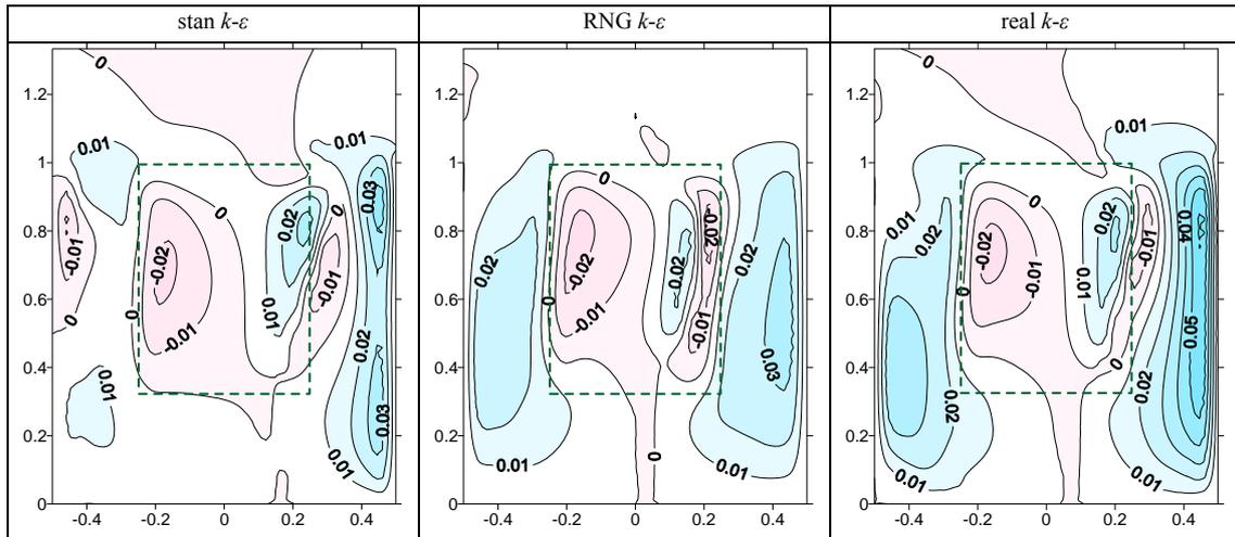
Figure 3. Normalized differences  $\Delta U_3/U_H$  (Equation 4) between simulations with the full set of vegetation terms (Equation 1-3) and the extra terms in the momentum equations only (Equation 1).
