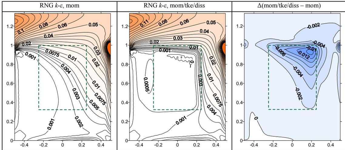
Figure 5. Normalized dissipation rates  $\varepsilon H/U_H^3$  for the RNG  $k-\varepsilon$  turbulence model simulations.
