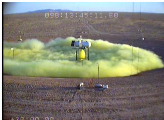
Figure 1. Trial 2-PC chlorine cloud, at 22 s after the release began.
