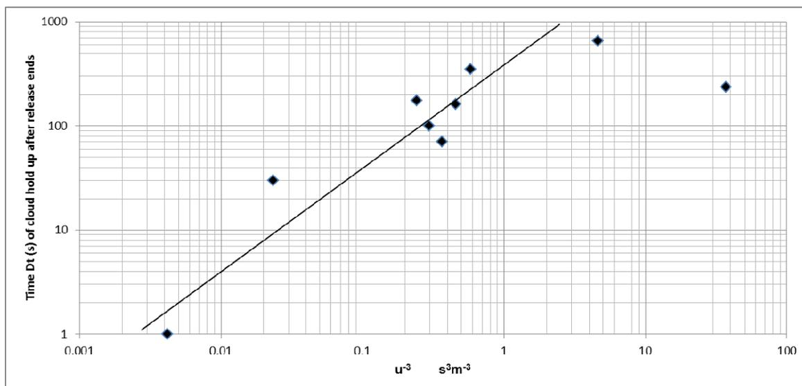
Figure 2. Scatter plot of observed cloud hold-up time  $Dt$  versus  $1/u^3$  for nine JR trials (from Table 1). A straight line,  $Dt = 350 u^{-3}$  provides a good fit to these points and is consistent with the power law suggested by Briggs et al. (1990).
