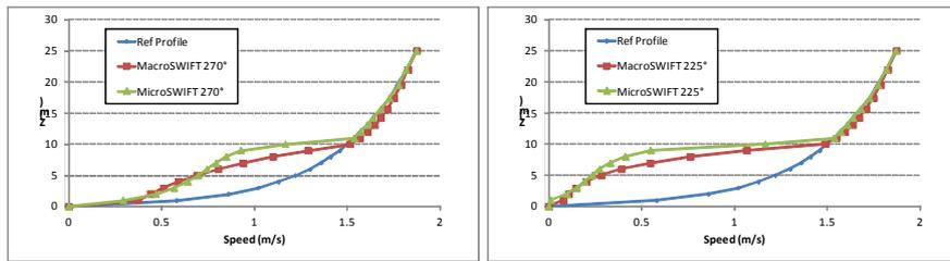
Figure 3. Vertical profiles of horizontal wind velocity – Free flow (blue) / Micro SWIFT explicit buildings (green) / SWIFT directional urban canopy (red) – Main flow direction aligned with cube arrays (left) / 45° off cube array direction (right).
