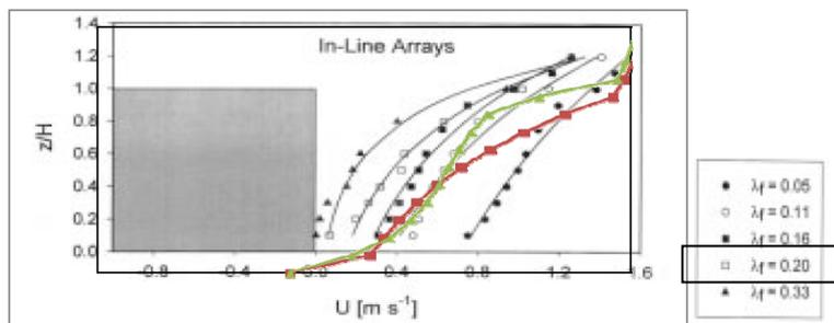
Figure 4. Vertical profiles of horizontal wind velocity – Spatial average of wind tunnel measurements for different  $\lambda_f$  (black and white dots) / SWIFT for  $\lambda_f=0.16$  with explicit buildings (green) and directional urban canopy (red)
