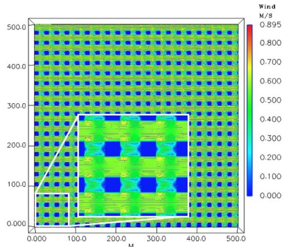
Figure 2. Horizontal slice for the wind speed and flow streamlines of the case  $\lambda_f = 0.16$  for Micro SWIFT
