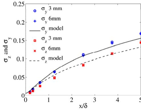
Figure 3. Vertical and lateral plume spreads from experimental data and comparison with the model (Eq. 1).
