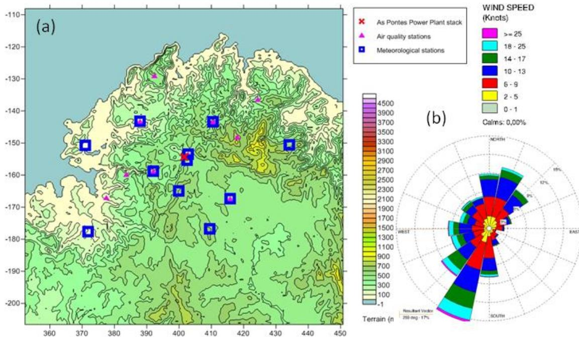
Figure 2. Surrounding area around As Pontes Power Plant stack (X), also showing: (a) meteorological and air quality sites; (b) typical annual wind rose in this region.
