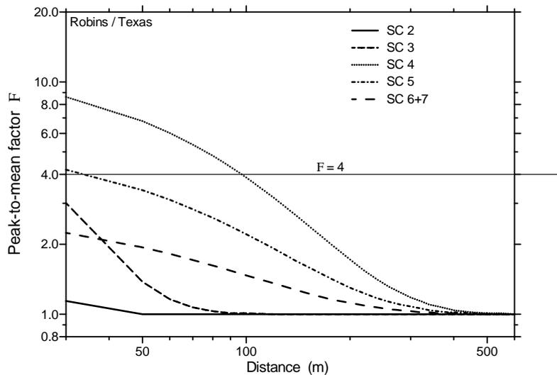
Figure 1 Distance depending peak-to-mean factor  $F$  for all stability class used by the AODM. The constant factor  $F = 4$  applied by AUSTAL2000 is shown as a thin straight line (source: Piringer and Schaubberger (2013)).
