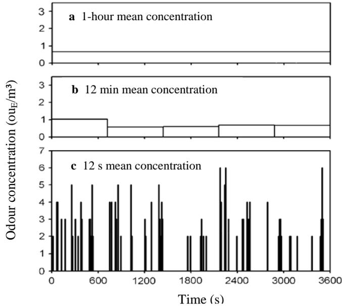
Fig. 1: Time course of the odour concentration (ouE/m<sup>3</sup>) for three time intervals. (a) one-hour mean value (e.g. output of a dispersion model), (b) 12-min and (c) 12-s mean odour concentrations observed at a single receptor point during a field study. The 12-s mean values were recorded and subsequently used to calculate 12-min and one-hour mean concentrations (source: Schauburger et al. (2012), modified from Nicell (2009)).
