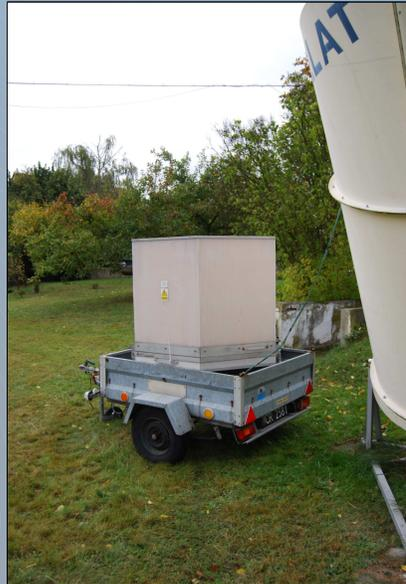
Mobile vertical monostatic Doppler SODAR, model 1DDS – the tool for acoustic sounding of atmospheric boundary layer.
