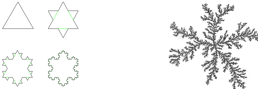
Figure 21: Left: first 4 iterations of the Koch snowflake curve. The length of this curve is (4/3)^N , where N is the number of iterations.. Right: Diffusion limited aggregation snow/fern like structure. ( http://classes.yale.edu/fractals/panorama/Physics/DLA/DLA.html )
