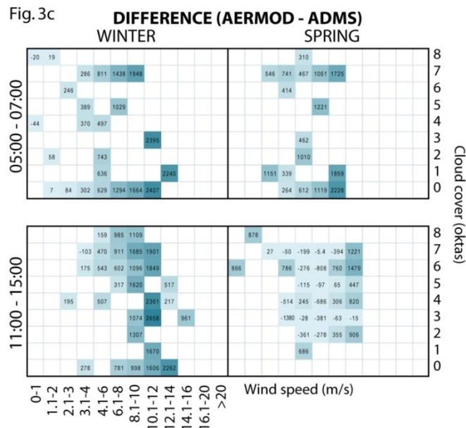
Fig. 3 Sub-sections of Dispersion Calendars showing means values of modelled boundary-layer height for ADMS (a) and AERMOD (b). The Calendar in (c) shows the difference in boundary-layer height, calculated as AERMOD (b) – ADMS (a).
