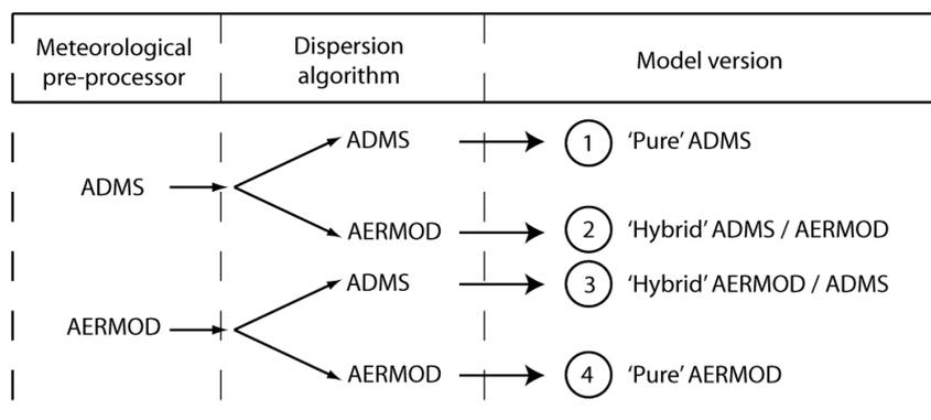
Fig. 1 The hybrid model of ADMS and AERMOD. Pathways show how users can combine meteorological and dispersion components of each model
