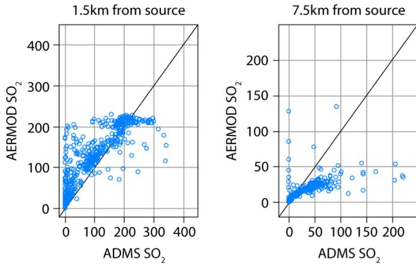
Fig. 2 A comparison of modelled SO<sub>2</sub> impacts from ADMS and AERMOD for near- and far-field receptors (1.5 and 7.5km) and convective conditions ( $H/L_{MO} < -0.3$ ). Source modelled is a stack of height 150m and diameter 4m. SO<sub>2</sub> is emitted at a constant rate of 1000g/s, with an exit temperature of 130 degrees C and exit velocity of 25m/s.
