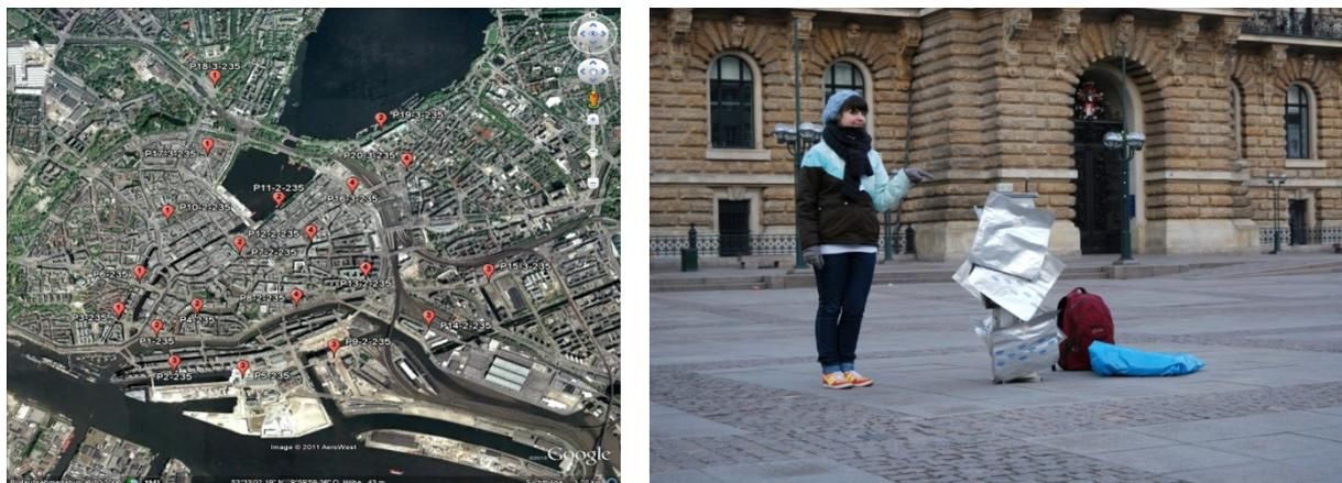
Fig 3: (a) Measurement positions during the field experiments and (b) picture of an automated bag sampler rig in front of the Hamburg town hall.
