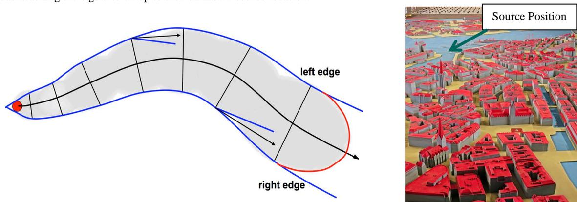
Fig. 2: (a) Top view on a plume dispersing in an environment in which obstacles effect plume shape and direction. The left and right plume edges are determined from the mean and turbulent velocity field computed by the LES model in a narrow 2.5m grid. (b) Geometrical detail of the physical model of Hamburg in the wind tunnel and indication of the source position during the field tests.
