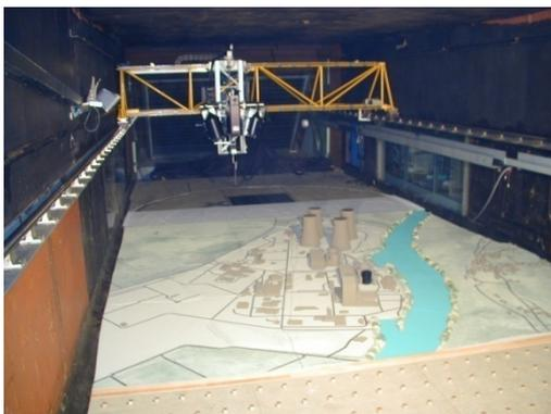
Figure 1. Bugey model in LMFA test section
