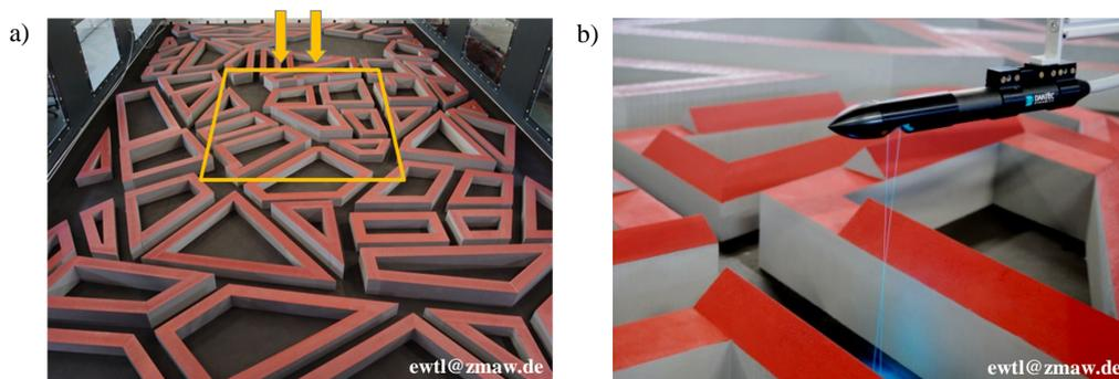
Figure 1. (a) Wind-tunnel model of semi-idealized complexity. The rectangle encompasses the model region of densely spaced flow measurements. The arrows indicate the inflow direction. (b) Optical flow sensing inside a street canyon with an LDV probe.
