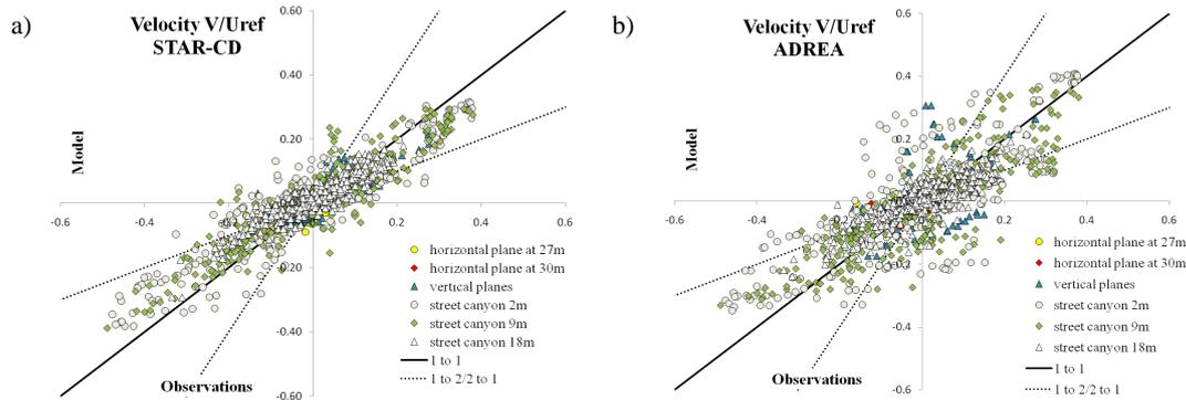
Figure 3. Scatter plots of measured versus modelled spanwise velocities from (a) STAR-CD and (b) ADREA.
