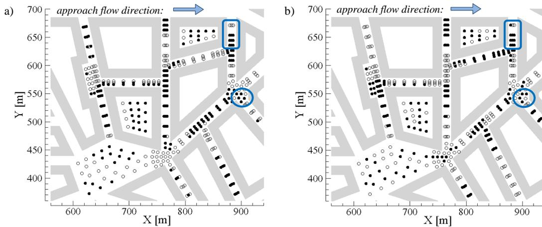
Figure 4. Local FAC2 distribution of the streamwise U (a) and spanwise V (b) velocity components as calculated from ADREA at a height of 2m. Black dots mark locations where  $FAC2 \leq 0.5$  and white dots where  $FAC2 > 0.5$ .
