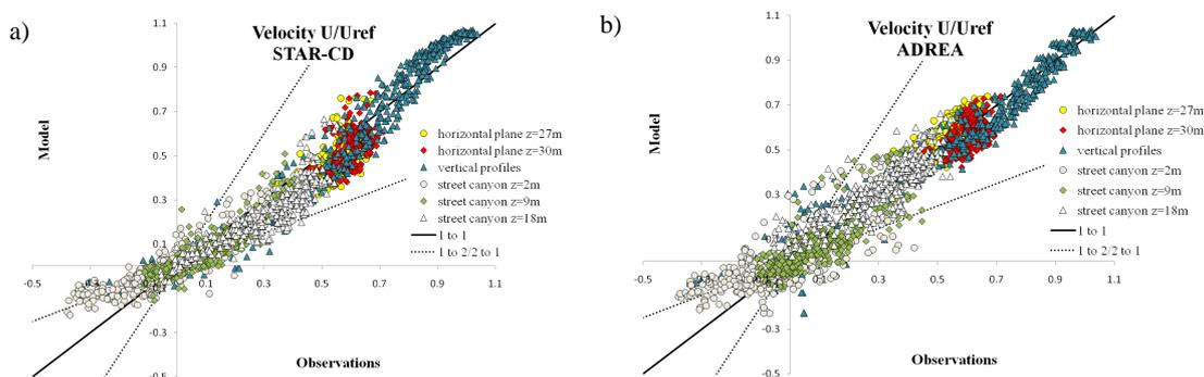
Figure 2. Scatter plots of measured versus modelled streamwise velocities from (a) STAR-CD and (b) ADREA.
