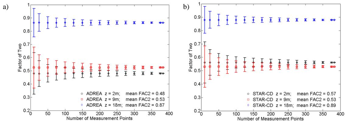
Figure 5. Dependence of the FAC2 of the streamwise velocity component  $U/U_{ref}$  at street canyon level on the number of measurement points used for its calculation: (a) for ADREA predictions and (b) for simulations with STAR-CD.
