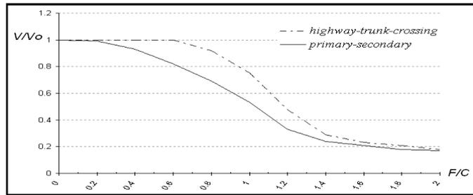
Figure 2. Speed functions ( $v/v_0$ : real versus free-flow speed ratio;  $F/C$ : traffic flow versus road capacity)
