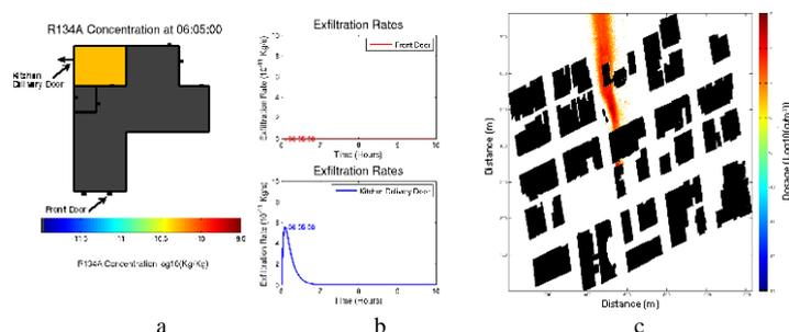
Figure 21. The output from the CONTAM interior and QUIC exterior “building-aware” dispersion models. The images depict the interior contaminant concentration and direction of material flow (a), the exfiltration rates through the front and kitchen delivery doors (b), and the exterior contaminant dispersion (c) for the weather conditions from node 190.
