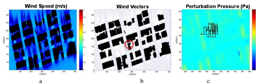
Figure 20. The output from the QUIC modelling system for SOM node 190 for wind speed (a), wind direction vectors (b), and perturbation pressure (c). The dots in figure c correspond with infiltration/exfiltration points that correspond with the configuration of the CONTAM interior dispersion model.
