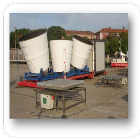
Figure 28. RASS/Sodar station with the Sonic Anemometer.
