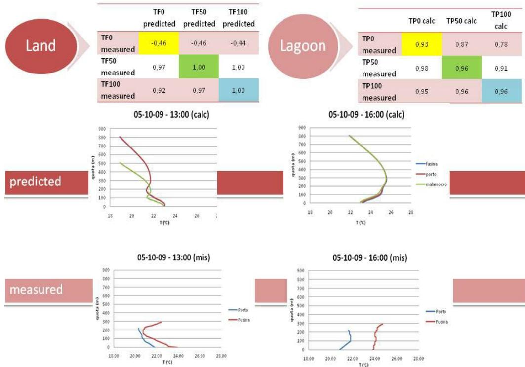
Figure 31. Comparison between predicted and measured data, land – lagoon case.
