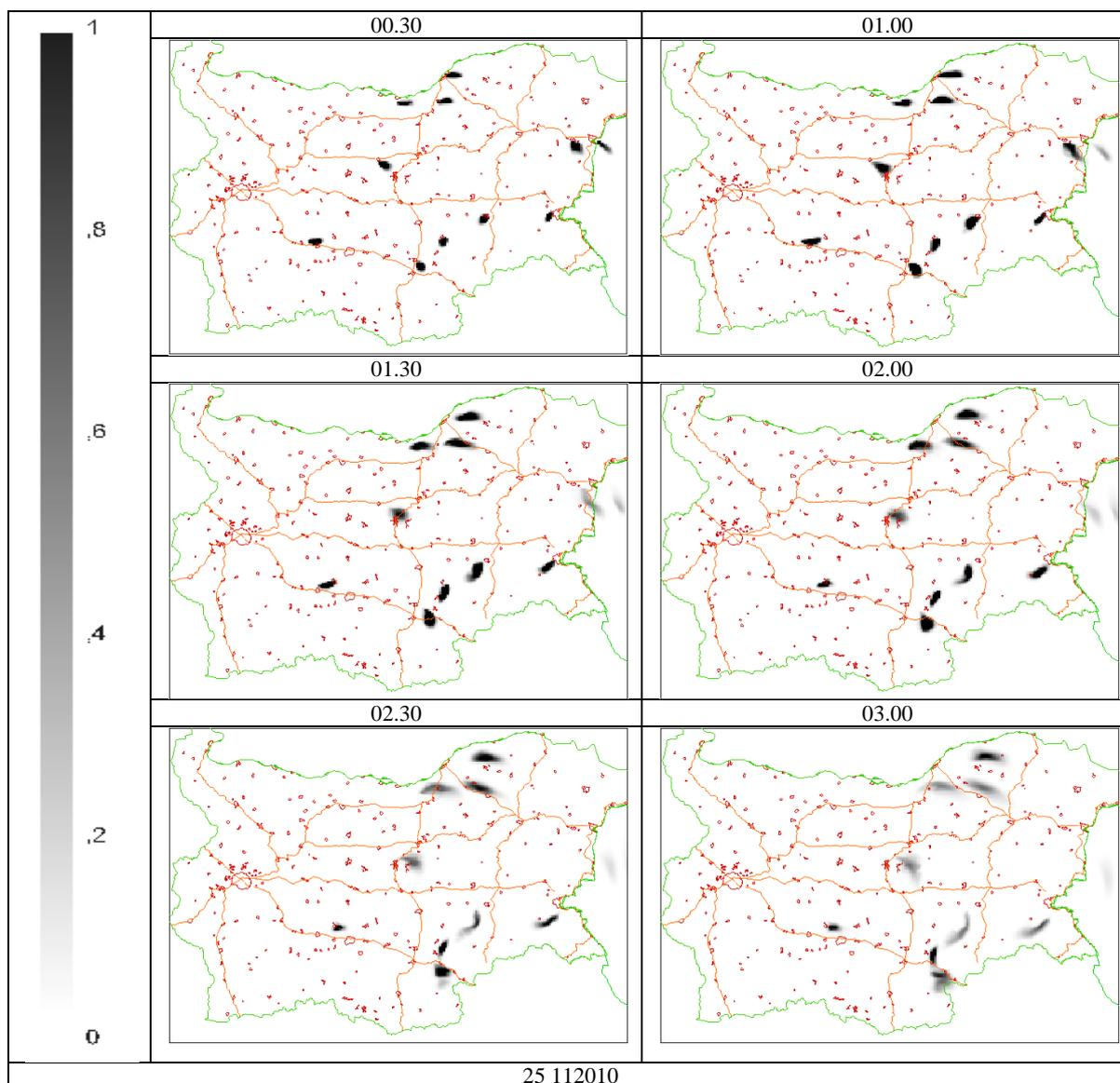
Figure 3. 3-hour tracer evolution for release at 0 o'clock on 25.11.2010.
