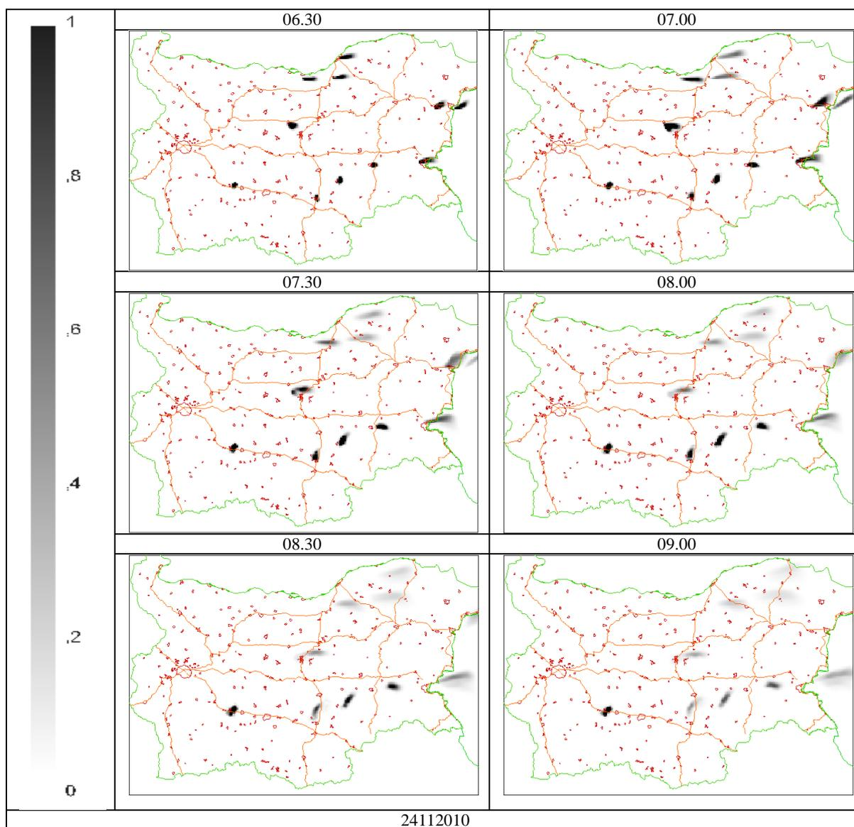
Figure 2. 3-hour tracer evolution for release at 6 o'clock on 24.11.2010.
