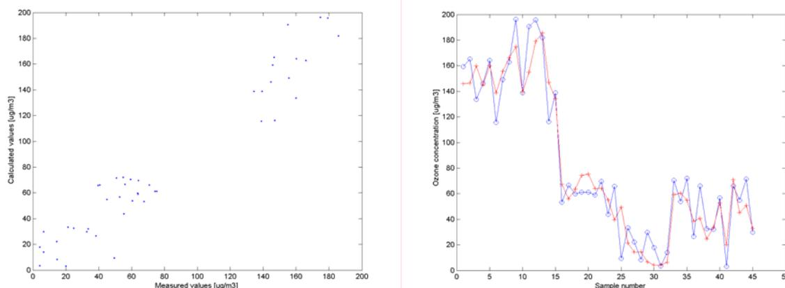
Figure 3. FL model: scatter plot and time series of forecasted ozone values for the verification set
