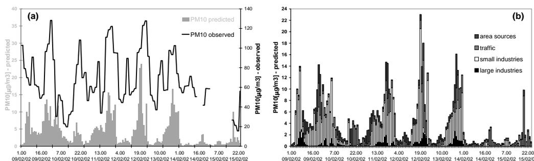
Figure 3. Modelled vs measured data for PM10 (a) and relative sources contribution (b)
