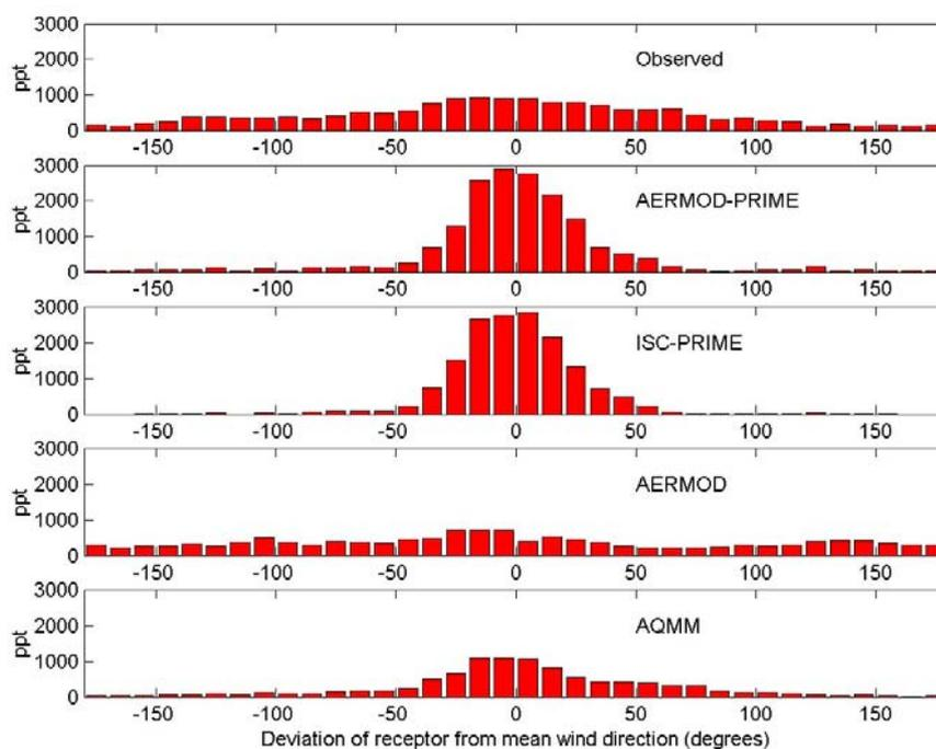
Figure 1. Concentrations as a function of the deviation of the wind direction from the line joining the centre of the source to the receptor.
