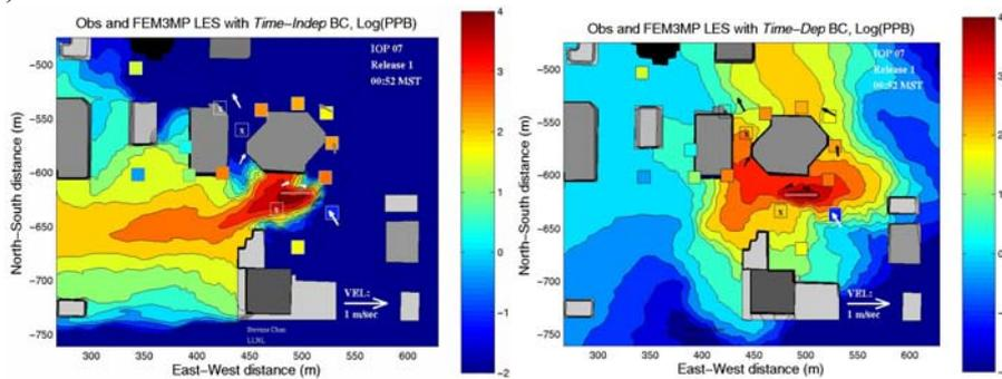
Figure 3. Predicted five minute time-averaged concentration patterns from simulations using steady-state (left) and time-dependent (right) inlet velocity component (URBAN 2000 data).
