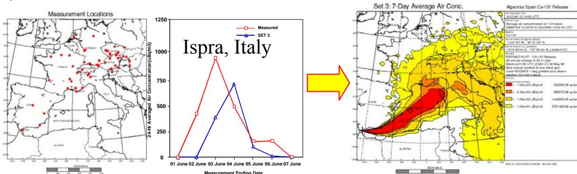
Figure 4. Manual event reconstruction example performed by NARAC for an accidentally melted medical source in Algeciras, Spain. Figure shows data locations (left), a model-data comparison for one location (middle), and the best NARAC prediction (right).
