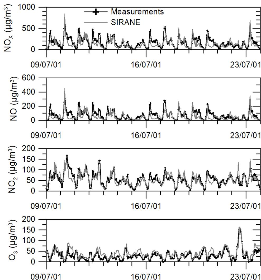
Figure 3. Comparison between SIRANE model and field measurements performed in Garibaldi Street.  $\text{NO}_x$ ,  $\text{NO}$ ,  $\text{NO}_2$  and  $\text{O}_3$  concentrations during the 15 days of the LYON6 campaign.
