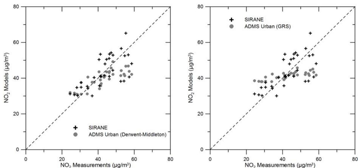
Figure 2. Comparison between SIRANE, ADMS Urban and field measurements performed with passive diffusion tubes.
