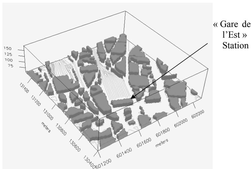
Figure 1. Domain 1100 m x 1100 m x 170 m with a mesh 10m in horizontal and a stretching mesh in vertical from 1 m close to the ground to 40 m at the top of the domain.
