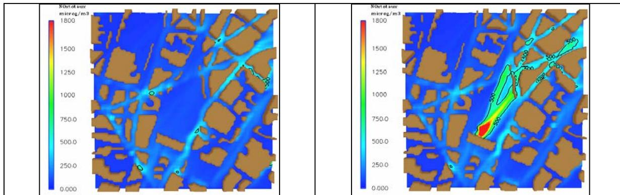
Figure 3. NOx concentration (wind 5 m/s SW) left : without Diesel locomotives right: 6 minutes after locomotives engines running (with  $500 \mu\text{g}/\text{m}^3$  isocontour)
