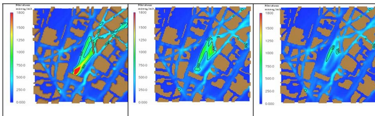
Figure 5. Impact on air quality 6 minutes after engine starts: from left to right, 1) old engines 2) new warming up protocol (reduced from 6 to 2 minutes) 3) new motorization of engines.
