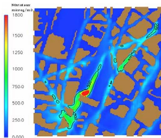
Figure 4. NOx concentration (wind 5 m/s NE): 6 minutes after locomotives engines running (with  $500 \mu\text{g}/\text{m}^3$  isocontour)
