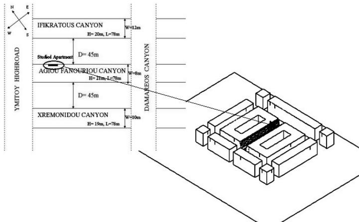
Figure 1. Ground plan of solution domain and corresponding numerical model
