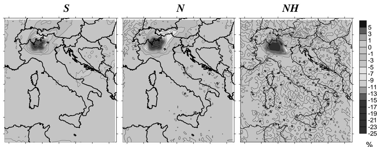
Figure 4. Changes in deposition of sulphur (left), oxidised nitrogen (centre) and reduced nitrogen (right) as a consequence of 25% reduction of emissions of  $SO_x$ ,  $NO_x$  and  $NH_3$ , respectively, in the Lombardy region (total deposition in a winter week)
