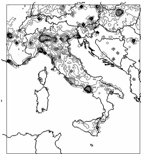
*Figure 3. Example of ground level NO<sub>2</sub> concentrations, computed for October 1, 1999, 19 UTC ( isolines every 5 ppb)*
