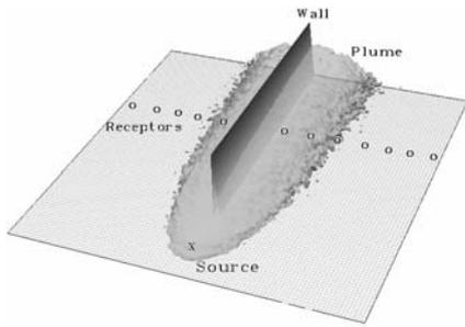
**Figure 2: Calculation domain for case #1. Wind velocity 5 m.s<sup>-1</sup>. Neutral atmosphere.**
