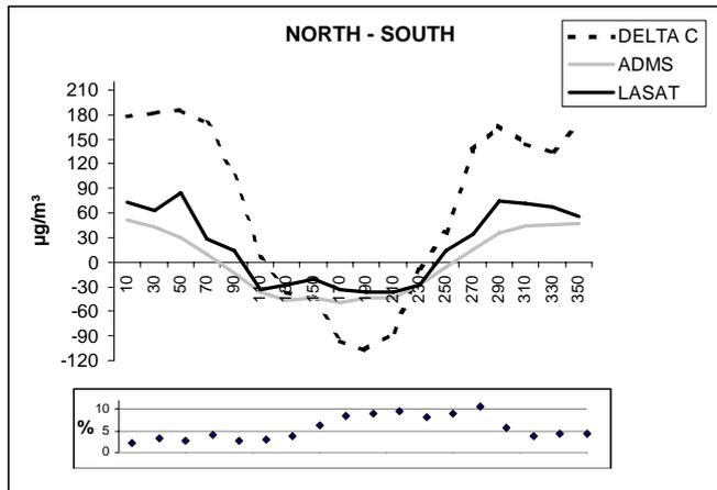
Fig.3; Differences between calculated north- and southside NO<sub>x</sub> concentrations compared to the measurements. The wind direction frequency (%) is shown at the bottom. The concentrations are averaged for wind sectors of 20°.
