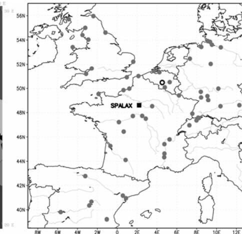
Figure 2: Location of the SPALAX detector and major potential sources identified in the calculation domain (circle: European NPPs; ring: medical isotopes facility).
