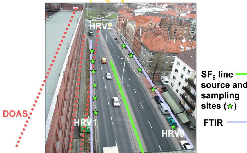
Fig.1: Street Canyon 'Goettinger Strasse' with instrumentation. The picture shows the continuous monitoring stations HRV1 to HRV3 in white and the SF<sub>6</sub>-line-source at the median strip plus the sampling bag locations in green colour. The path-averaged measurements are indicated by the blue solid (FTIR) and red dotted (DOAS) lines.
