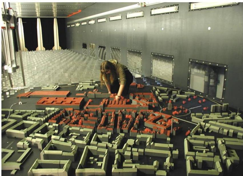
Fig. 2: Physical model of the site in the Boundary Layer Wind Tunnel of Hamburg University
