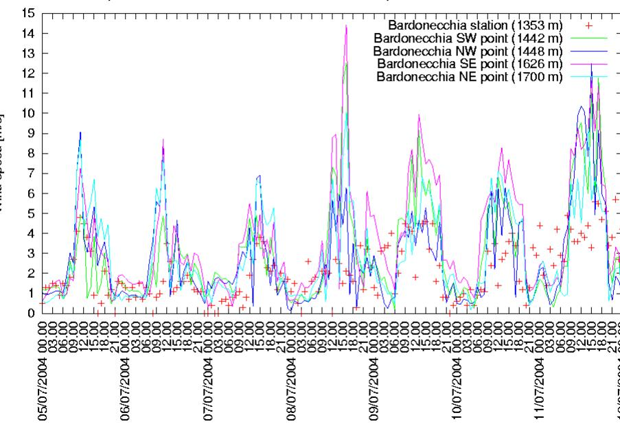
Comparison between measured and simulated wind speed (MINERVE) - Bardonecchia 5-11/07/2004
